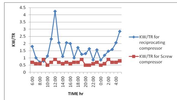
Figure 11 Graph between specific power KW/TR and TIME hr
