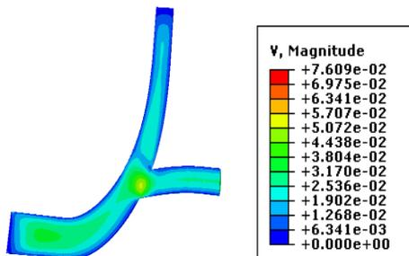
Figure 8 Contour plot of Velocity (Magnitude) for Newtonian blood with ramp amplitude (Uniformly decreasing)
