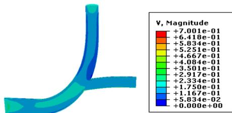
Figure 11 Contour plot of Velocity (Magnitude) for Newtonian blood with modulated data
