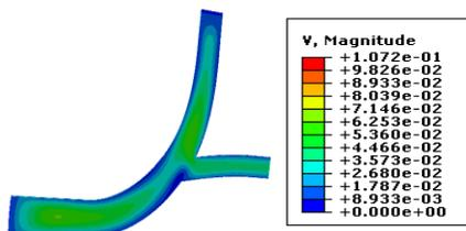
Figure 12 Contour plot of Velocity (Magnitude) for Newtonian blood with exponential decay
