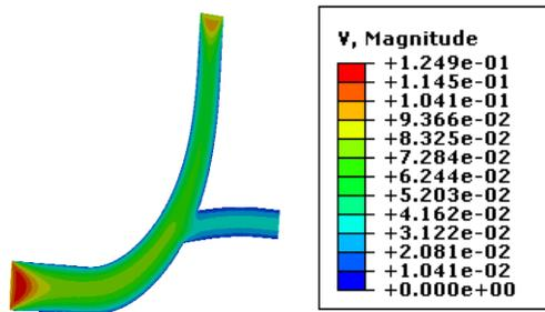
Figure 7 Contour plot of Velocity (Magnitude) for Newtonian blood with ramp amplitude (Uniformly increasing)
