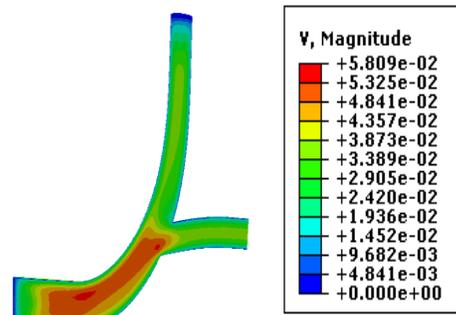
Figure 9 Contour plot of velocity (Magnitude) for Newtonian blood with ramp amplitude (Variable)
