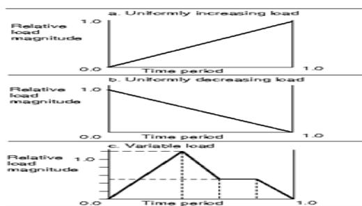
Figure 1 (a-c) (a) Ramp with uniformly increasing load
