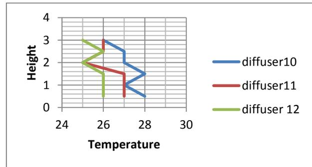
Graph.2 Variation in temperature vs. height at location X1 with load 1500W
