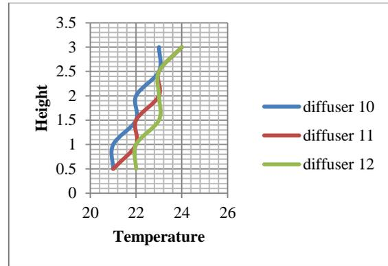
Graph.11 Variation in temperature vs. height at location X1 in condition 1 without load
