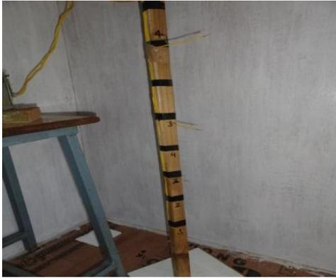
Figure 8 Air temperature measurement with thermocouple
