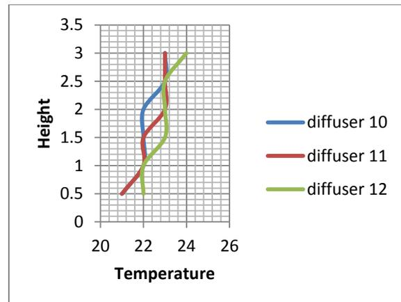
Graph.13 Variation in temperature vs. height at location X2 in condition 1 without load
