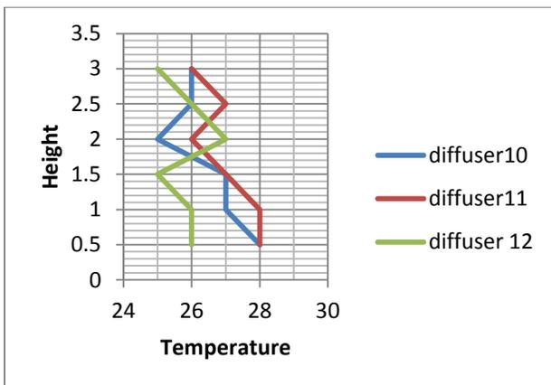
Graph.6 Variation in temperature vs. height at location X3 with load 1500W
