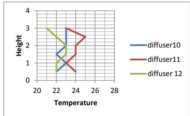
Graph.3 Variation in temperature vs. height at location X2 without load
