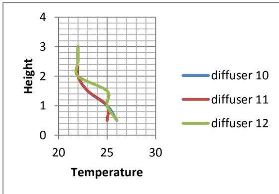
Graph.16 Variation in temperature vs. height at location X3 in condition 1 with load 1000 W
