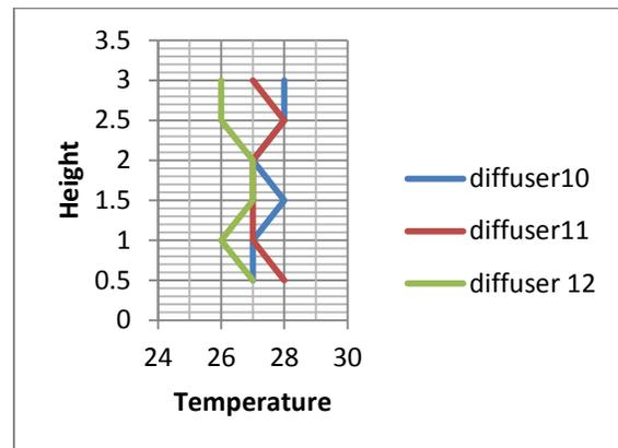
Graph.8 Variation in temperature vs. height at location X4 with load 1500W
