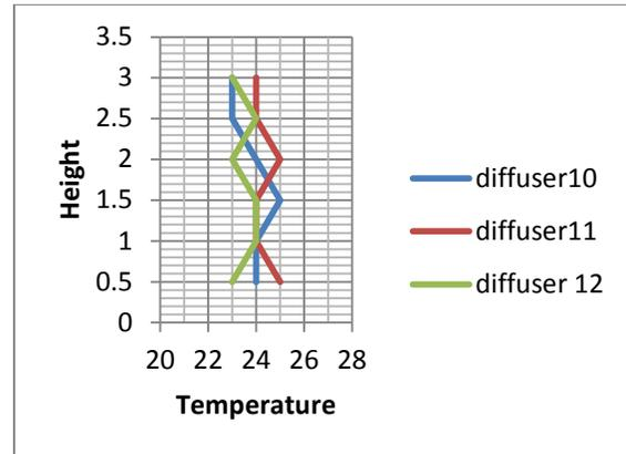
Graph.7 Variation in temperature vs. height at location X4 without load
