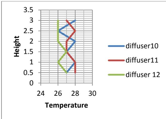
Graph.4 Variation in temperature vs. height at location X2 with load 1500W
