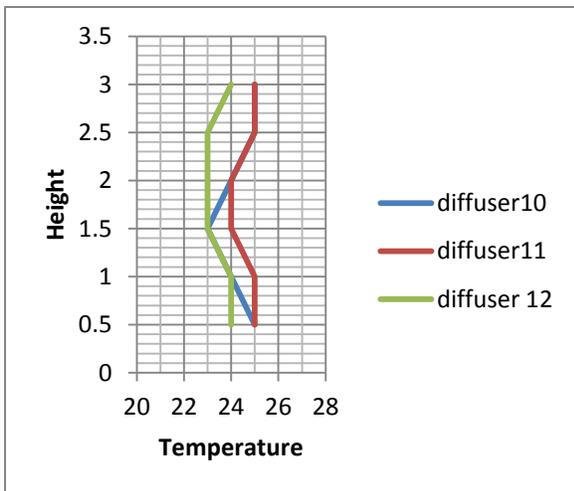
Graph.5 Variation in temperature vs. height at location X3 in without load
