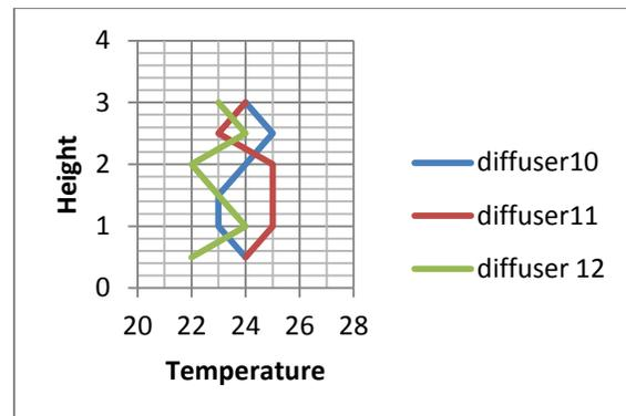
Graph.9 Variation in temperature vs. height at location X5 without load
