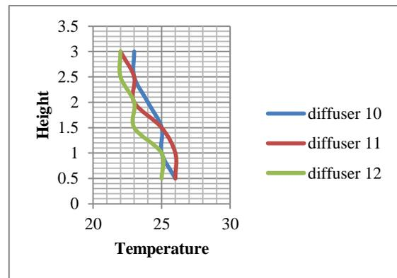
Graph.18 Variation in temperature vs. height at location X4 in condition 1 with load 1000 W
