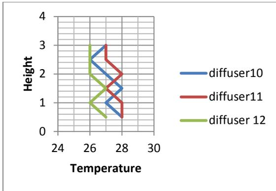
Graph.10 Variation in temperature vs. height at location X5 with load 1500W
