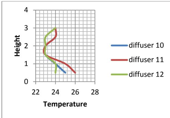
Graph.14 Variation in temperature vs. height at location X2 in condition 1 with load 1000 W
