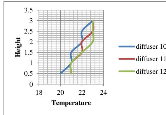
Graph.19 Variation in temperature vs. height at location X5 in condition 1 without load
