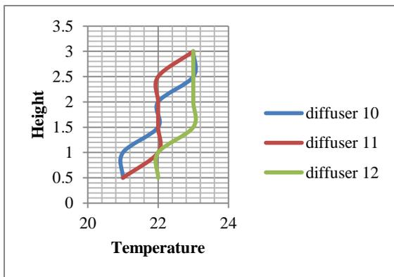
Graph.15 Variation in temperature vs. height at location X3 in condition 1 without load
