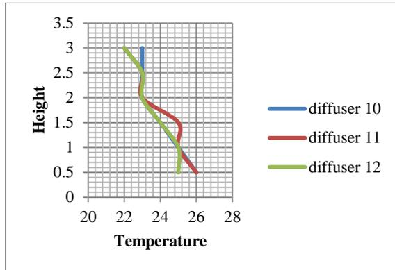
Graph.20 Variation in temperature vs. height at location X5 in condition 1 with load 1000 W
