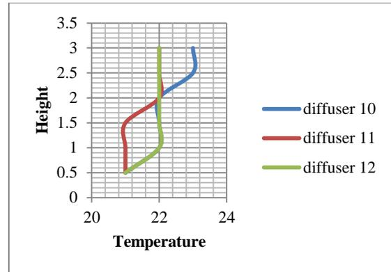
Graph.17 Variation in temperature vs. height at location X4 in condition 1 without load
